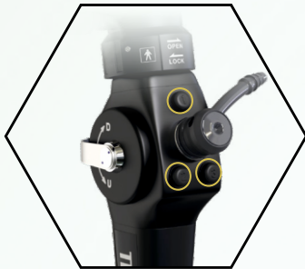
Multi-function Buttons ①Zoom ②Capture/Record ③Freeze
